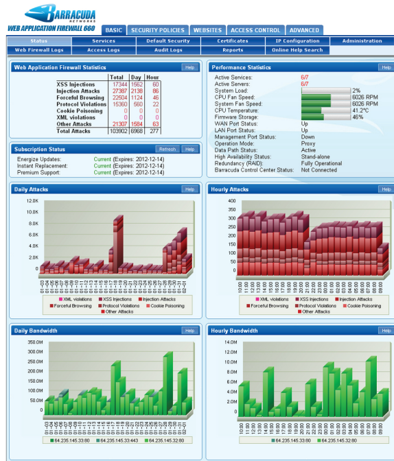
The Barracuda Web Application Firewall Vx monitors and tracks common application attacks, performance statistics and bandwidth usage.
